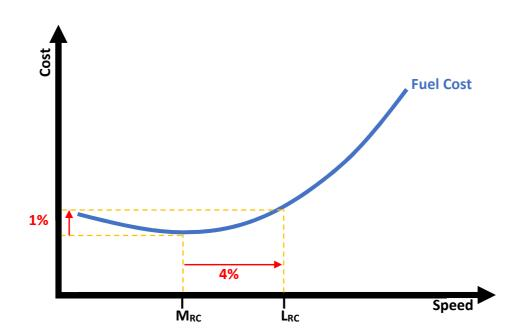
The advantage of flying at the maximum range speed is simply that the aeroplane will use the least amount of fuel and therefore have the least fuel cost for a given distance. However, operationally, the faster "long range cruise" is used. The simple reason why this speed is used is because by getting to destination more quickly; more revenue earning flights can be carried out in any given period.
