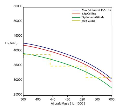
Therefore, to constantly fly at the optimum altitude, the aeroplane will not actually fly level, but will in fact slowly be climbing in the cruise. On the other hand, ATC restrictions require level flight cruise to ensure vertical separations with other aeroplanes. To try an accommodate ATC in congested airspace aircraft must fly by segments of constant altitude which must be as close as possible to the optimum altitude.
