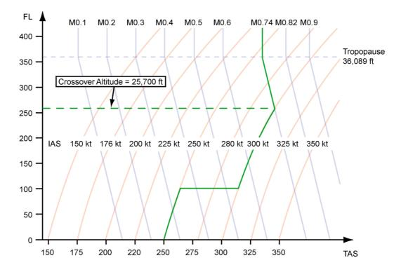
If a faster indicated airspeed climb is maintained, the crossover altitude is lower
