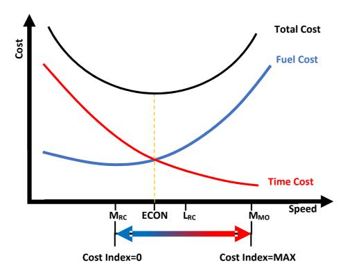
The total cost curve that the speed which gives the minimum total operating cost is the most economical speed to fly. This speed is called ECON, or the Minimum Cost Speed. The value of the ECON speed is worked out by the FMS based upon the value of the cost index. As a formula the cost index is a ratio of cost of time (CT) divided by the cost of fuel (CF).
