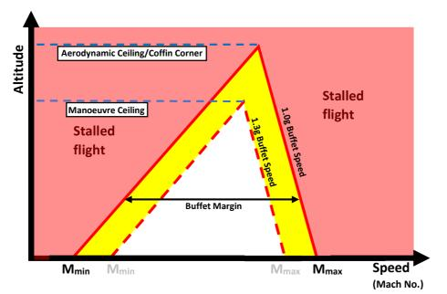
Taking into consideration both the Mach number for low speed and high speed buffet, it means that there are two mach numbers, below and above which the aeroplane is unable to fly. This speed range between the Mach number for the low speed stall and high speed stall is called **the buffet margin**.
