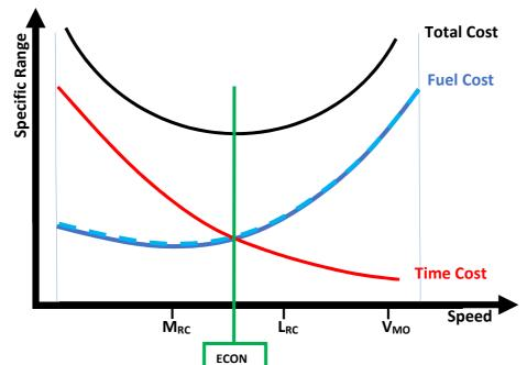
To summarise then, increasing the cost index from zero to maximum will increase the ECON speed from the maximum range speed to maximum operating speed. For most aeroplanes the cost index varies from 0 to 99 or from 0 to 999.
