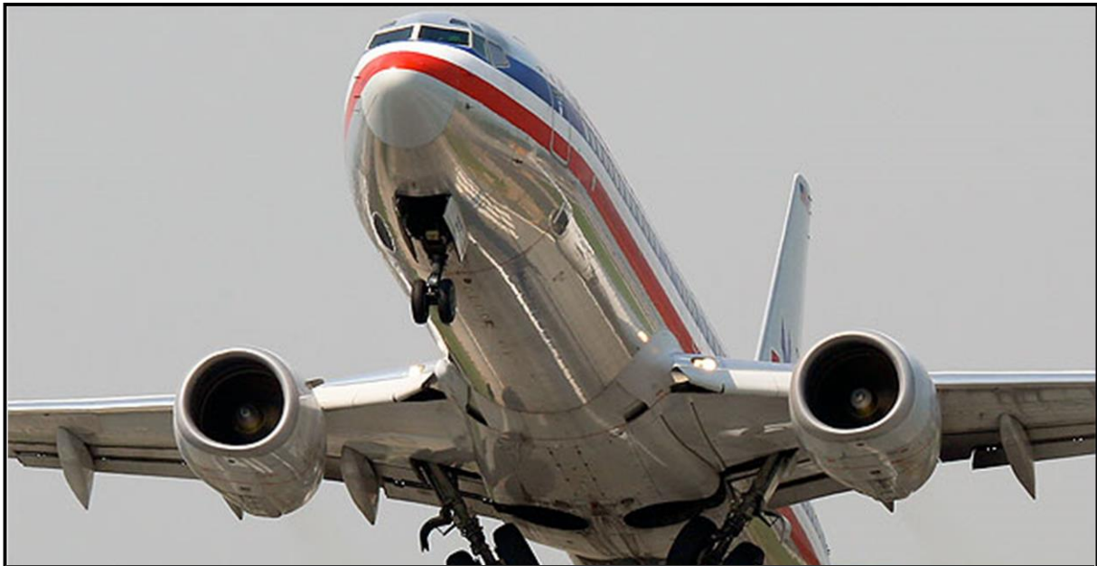
American Airlines Boeing B737 – Nose Landing gears rotating forward during retraction
