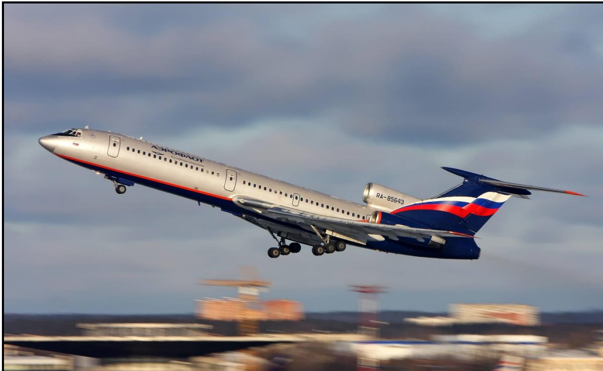
Aeroflot Tupolev TU154 – Nose Landing gears rotating afterward during retraction
