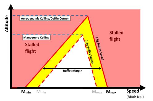
Taking into consideration both the Mach number for low speed and high speed buffet, it means that there are two mach numbers, below and above which the aeroplane is unable to fly.
