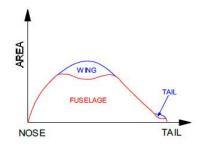
There is an optimum area distribution, and the minimisation of transonic interference drag requires that the aircraft should be designed to fit this distribution as closely as possible. This requirement is known as the **"area rule"**. In practice, no aircraft has this optimum distribution, but any reasonably smooth area distribution helps to reduce the transonic drag rise.
