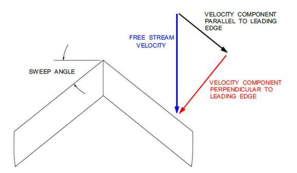
Sweeping the wing back has nearly the same aerodynamic advantages as a thin wing, without suffering reduced strength and fuel capacity.
