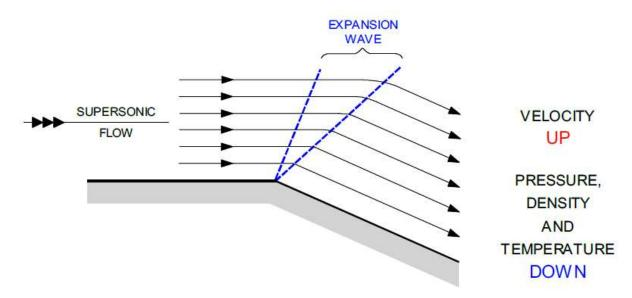
On the illustration above, it can be seen that a supersonic airflow can follow a convex corner because it expands upon reaching the corner. The velocity INCREASES and the other parameters, pressure, density and temperature DECREASE. Supersonic airflow behaviour through an expansion wave is exactly opposite to that through a shock wave.
