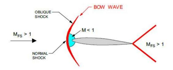
At an aircraft's M>1.0, The shock wave ahead of the leading edge is normal only in the vicinity of the leading edge, and oblique further away from the leading edge ("above" and "below"). This is called a **BOW SHOCKWAVE**
