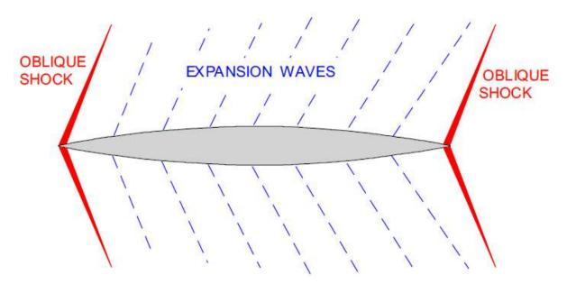
The figure above shows a series of expansion waves in a supersonic airflow. After passing through the bow shock wave, the compressed supersonic flow is free to expand and follow the surface contour. As there are no sudden changes to the airflow, the expansion waves are NOT shock waves.
