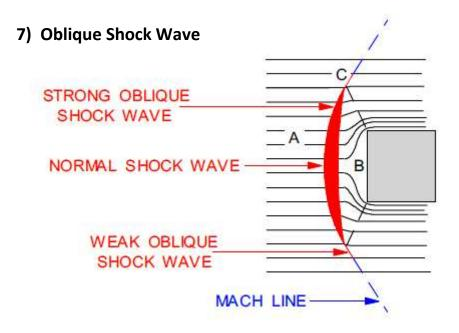
An oblique shock wave is a slightly different type of shock wave.
