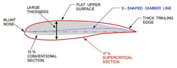
Because the airflow does not achieve the same increase of speed over the flattened upper surface compared to a conventional section, the formation of shock waves is delayed to a higher  $M_{FS}$  and are much smaller and weaker when they do form.
