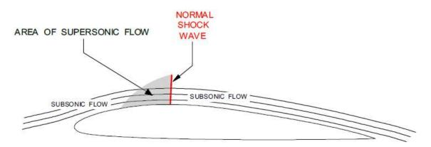
As the aircraft speed is further increased the region of supersonic flow on the upper surface extends and the shockwave marking the end of the supersonic region, moves rearwards. A similar sequence of events will occur on the lower surface although the shockwave will usually form at a higher aircraft speed because the lower surface usually has less curvature so the air is not accelerated so much.
