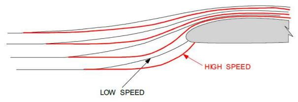
At a constant angle of attack, the increase of CL as speed increases from about M 0.4 into the low end of the transonic region gives a steeper lift curve slope, i.e. the change of CL per degree angle of attack will increase. However, because of earlier separation resulting from the formation of the shock wave,  $C_{LMAX}$  and the stalling angle will be reduced.
