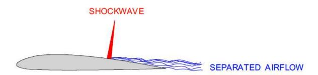
This is known as the **shock stall** because it results from a separated boundary layer just as the low speed stall does. The severity of the loss of lift depends on the shape of the wing sections. Wings not designed for high speeds may have a severe loss of lift at speeds above M<sub>CRIT</sub>, but wings designed specifically for high speed flight, with sweep back, thinner sections and less camber will have much less variation of lift through the transonic region.
