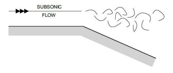
With subsonic airflow the adverse pressure gradient would be so steep that the airflow would instantly separate at the "corner".
