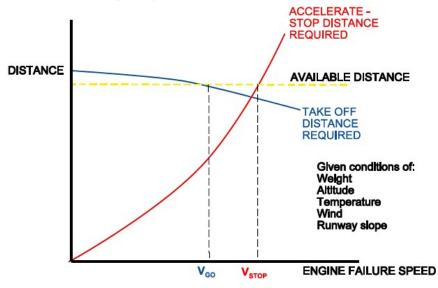
$V_{GO}$  is the first speed at which the take-off can be completed within the distance available.  $V_{STOP}$  is the last speed at which the accelerate-stop could be completed within the distance. The  $V_1$  speed can therefore be chosen anywhere between  $V_{GO}$  and  $V_{STOP}$ .
