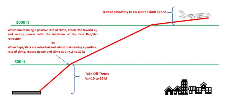
The two procedures differ in that the acceleration segment for flap/slat retraction is either initiated prior to reaching the maximum prescribed height or at the maximum prescribed height. To ensure optimum acceleration performance, thrust reduction may be initiated at an intermediate flap setting.
