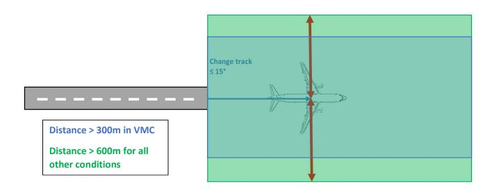
If the flight path requires track changes of more than 15°, obstacles need not be considered if the lateral distance is greater than 600m in VMC or 900m for all other conditions.
